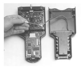
**5** Remove the retaining plate and keep the foam packaging for re-use.
