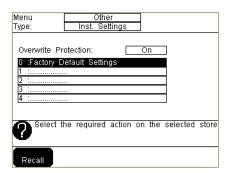
**2** Press Recall to recall the instrument default settings. The status display will indicate stored settings number 0 recalled.
